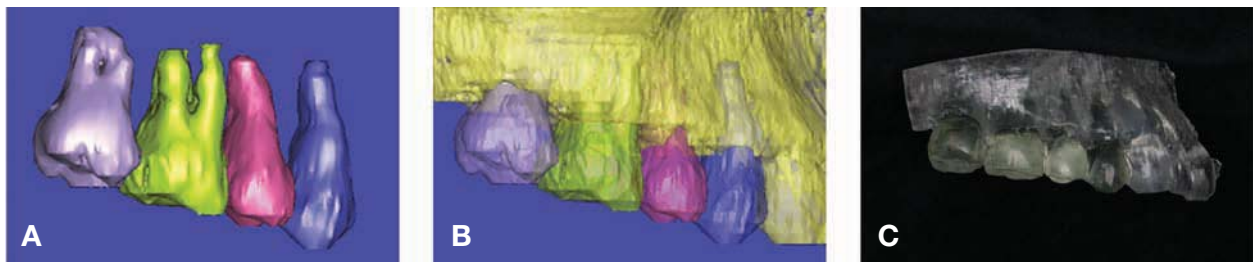
Fig 4. A and B, 3D imaging for replica model construction. C, Replica model using SLA method.
